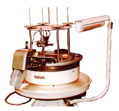
The machine is designed for linking the stockings extremity and berets (machine gauge: 10 E). The looping is performed by hooking up loop by loop on the fixed needles of the movable dial the two parts to be linked together. The looping is performed by elastic stitches with 2 yarns. The machine may be used for linking stockings or berets made of cotton or cotton-like yarns, wool- or silk-like man-made yarns.
